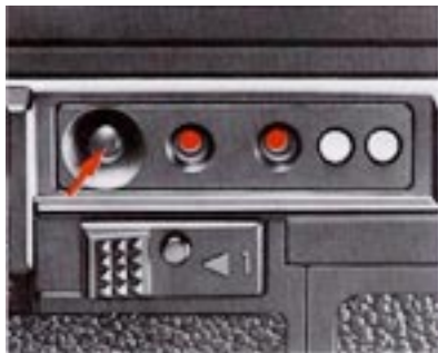
Battery Check Button(1) and LED Indicators(9)
